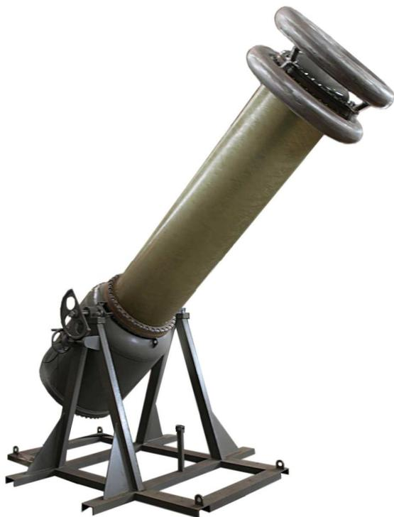
Single-phased gas-filled test transformer IOG-350-I (further on - transformer) is designed for testing high-voltage electrical equipment with short-term voltage of 50 Hz frequency, including tests with measuring insulation capacitance ( $C_X$ ), loss-angle tangent ( $\text{tg } \delta_{II}$ ) and partial discharges (PD).
